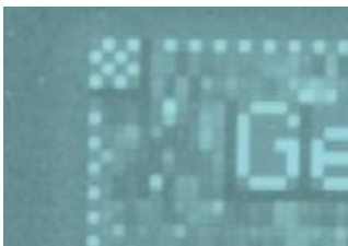
Figure1 : Fragment of DAT file, showing 4x4 checker-board used for alignment.
