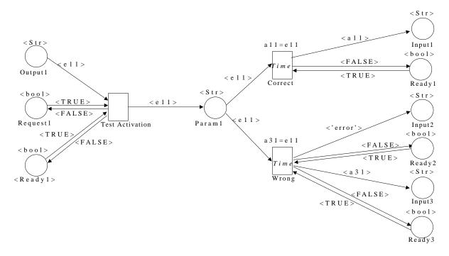
Figure 6: Pr/T net defining the job CheckDfd
