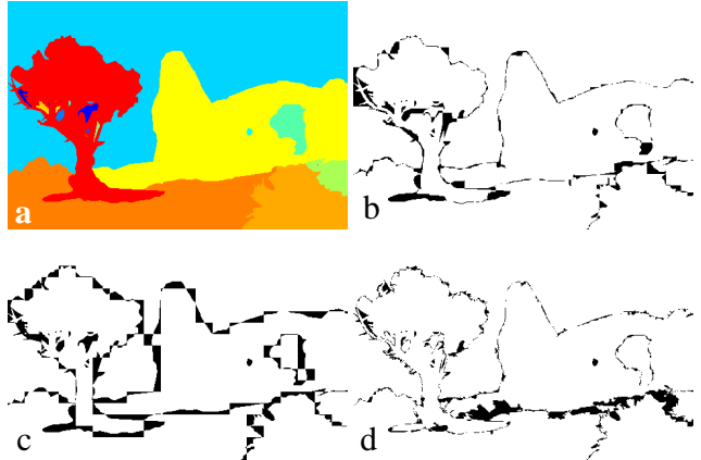
Figure 7. Accuracy of superpixels against human-labeled ground truth. a) Human-labeled ground truth regions. b) An example of the errors associated with the 20 \times 20 lattice presented in Figure 1b when compared to the ground truth in (a). Pixels in black will be misclassified by an ideal classifier as they lie in superpixels which are dominated by a different object class. c) Errors for uniform sampling. This can only produce piece-wise linear approximation to image boundaries. d) Errors for [3] with 400 superpixels.
