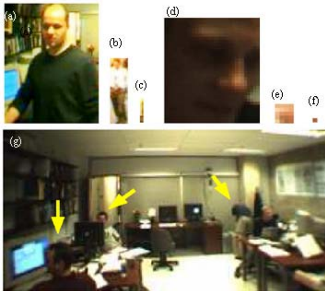
Figure 2: Conventional face/body detectors fail in the wide field image as pose variation and occlusion is too great, and many of the faces/bodies are very small. (a,b,c) show the largest ( 95 \times 78 pixels), median ( 52 \times 14 ) and smallest ( 15 \times 2 ) bodies identified by hand in a training set (d,e,f) show the largest ( 34 \times 31 ), median ( 5 \times 4 ) and smallest ( 1 \times 1 ) faces. Arrows in lower image depict other difficulties. From L to R, some people face away from the camera, others are partially occluded or are in unusual poses
