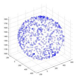
The values lie on (or close to the surface of) a sphere – which is good news, but the sphere isn't centred on zero, which is not. Note that, in some cases of magnetic interference, it is possible for the sphere to distort into an ellipsoid (something that looks more like an egg), which makes life just a little bit more problematic.
