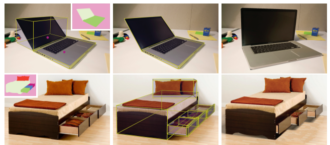
Figure 10: Users can provide high-level annotations: (top) the two proxies are marked to share a hinge joint; (bottom) the drawers are marked to be sliding inside the bed frame. Our framework computes the necessary joint attributes based on proxy geometry, making the images interactive (see the supplementary video and demo).
