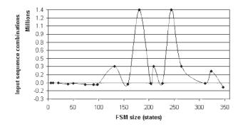
**FIGURE 6.** Difference in effort between worst case BFS and current GA results in attempt to find all UIOs of an FSM—four worst performing FSMs for BFS removed from graph.
