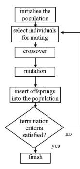
FIGURE 2. Flowchart for a basic GA.
