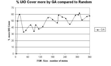
**FIGURE 11.** Percentage difference in UIOs generated by GA compared with random algorithm. Results for randomly generated FSMs.
