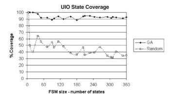
**FIGURE 10.** Percentage state coverage in UIOs generated by GA compared with random algorithm. The two GAs produced identical results. Results for randomly generated FSMs.
