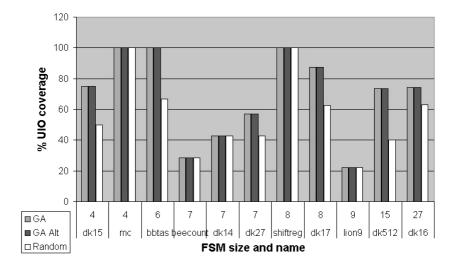
FIGURE 9. Percentage state coverage in UIOs generated by GA compared with random algorithm. Results for real FSMs.
