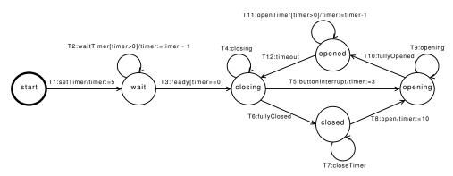
Figure 1. An EFSM specification for the door control of the elevator system.
