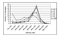
Fig. 5 Publish-subscribe model (32 hosts scenario): delivery ratio distribution of persistent messages vs buffer size.
