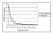
Fig. 2 Point to point model (32 hosts scenario): delay time distribution of persistent and non persistent messages.
