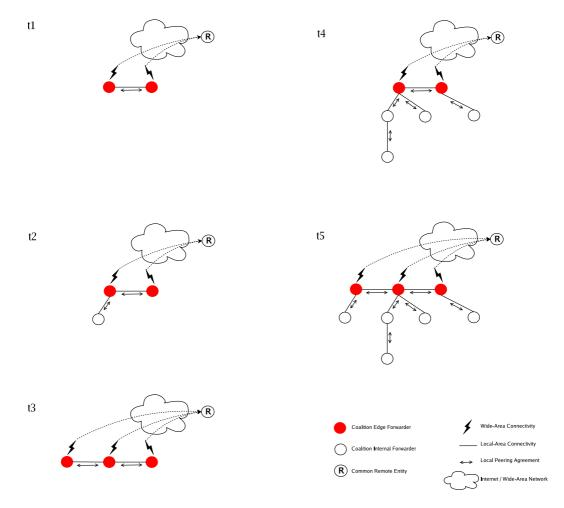
Figure 1: Experimental Network Topologies
