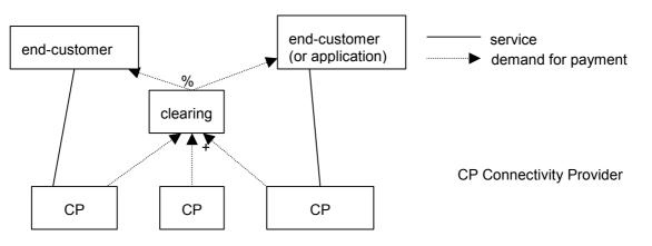
Figure 4.2: Clearing (distributed or not) among all connectivity providers in the communication
