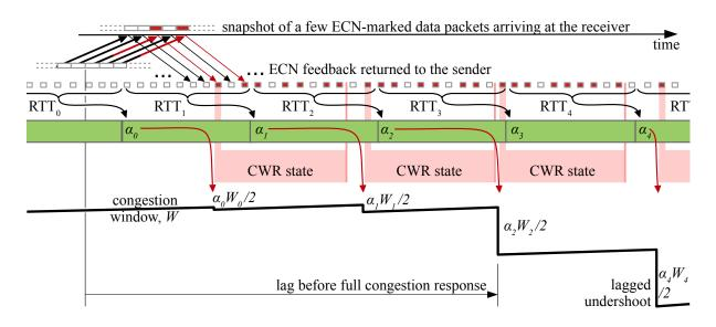
Figure 2: The problem: DCTCP's two stages for processing congestion feedback: 1) gathering feedback in a fixed sequence of rounds (RTT<sub>i</sub>) to calculate the EWMA ( $\alpha_i$ ); 2) applying this EWMA on the first feedback mark, when it has had no time to gather enough feedback, which leads to a typically inadequate congestion response before entering congestion window reduced (CWR) state, which suppresses any further response for a round. See text for full commentary.
