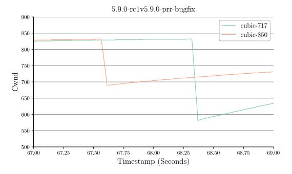
Figure 8: TCP CUBIC congestion window behaviour is also fixed (c.f. Figure 5). Excerpt of cwnd time sequence plot for two single flows using TCP CUBIC with beta parameter 717 (0.7) and 850 (0.83).
