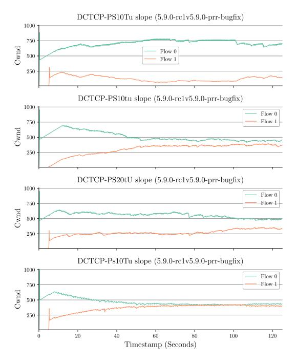
Figure 9: The latecomer disadvantage appears once the PRR bug is fixed. Time sequences of cwnd for two identical variants of DCTCP with starts staggered by 5 s (all with PRR fixed): i) regular DCTCP; ii) DCTCP without toggling to 0 of the EWMA; iii) DCTCP with upscaled EWMA and 20-bit precision; iv) DCTCP without TSO. Each affects two flow's ability to converge to equal rate to different degrees. Capacity: 200 Mb/s; RTT: 50 ms; AQM: step at 2 ms.
