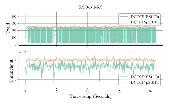
Figure 2: The Effect of the PRR bug in a Data Centre scenario. DCTCP with PRR (DCTCP-PS10Tu) suffers from lower utilization because it almost halts sending during recovery and it ends up sending larger bursts when compared with DCTCP without PRR (DCTCP-pS10Tu). Capacity: 5 Gb/s; RTT: 1 ms; AQM: step at 163 us.
