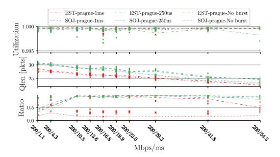
Figure 23: The same results as in Figure 21 showing that smaller burst size seems to fix the latecomer disadvantage, except fairness is shown as a simple rate ratio.
