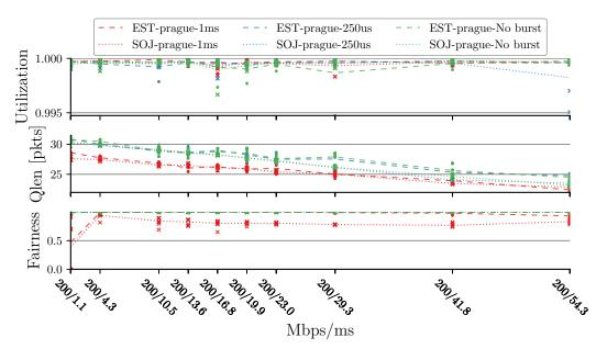
Figure 21: EST marking and lower burst size also seem to fix the latecomer disadvantage over a sweep of RTTs (the fairness plots for EST-prague-250 and for low or no TSO all overlap along the 1.0 fairness ceiling). The metrics and six combinations of set-up are the same as in Figure 20
