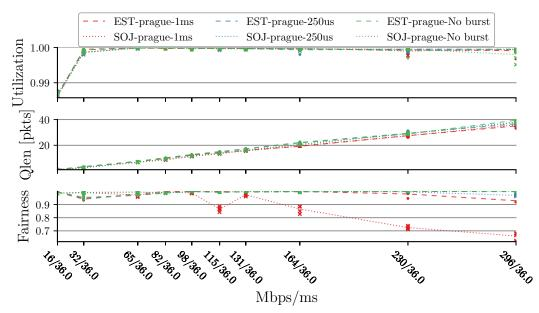
Figure 20: EST marking seems to fix the latecomer disadvantage over a sweep of linkrates, particularly in combination with reduced burst duration (the fairness plots for EST-prague-250 and TSO disabled all overlap along the 1.0 fairness ceiling). The plots show average utilization, queue length and fairness for the two delay metrics at the AQM (EST and sojourn time) and three different TSO burst sizes at the sender. Capacity: varied; RTT: 36 ms; AQM: step at 2 ms.
