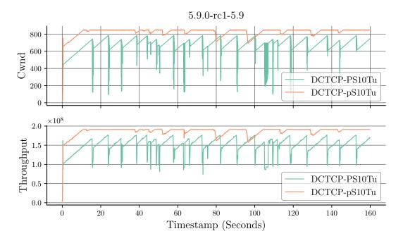
Figure 3: The Effect of the PRR bug in a Wide Area Network scenario is similar to that in the Data Centre scenario of Figure 2 Capacity: 200 Mb/s; RTT: 50ms; AQM: step at 1 ms.
