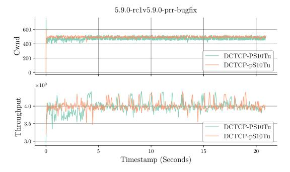
Figure 6: Fixed PRR bug in a data centre network scenario (c.f. Figure 2). Aligning Linux's implementation with RFC6937 fixes the PRR bug and its consequences.
