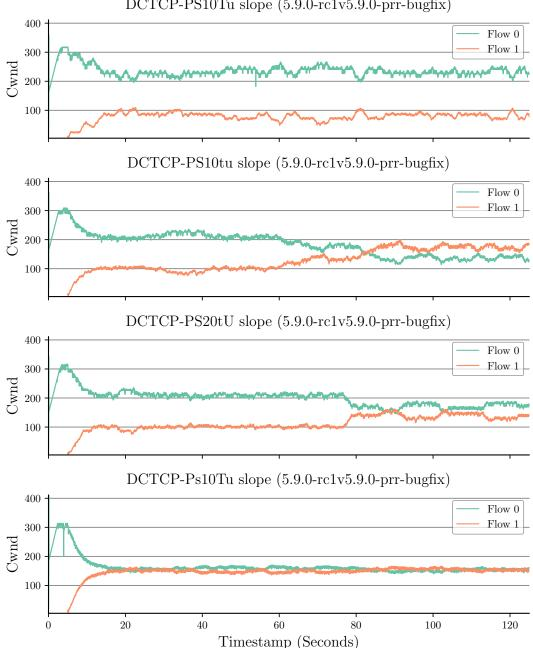
DCTCP-PS10Tu slope (5.9.0-rc1v5.9.0-prr-bugfix)
