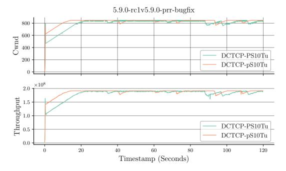
Figure 7: Fixed PRR Bug in a wide area network scenario (c.f. Figure 3). Aligning Linux's implementation with RFC6937 fixes the PRR bug and its consequences.
