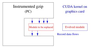
Fig. 1. The original code is instrumented to record the inputs and outputs (blue arrows) of the target function (red) every time it is called. These become the fitness function and test suite for the automatically evolved replacement module running on novel hardware (actually GPUs). The CUDA code generated by GP is functionally identical to the C code inside gzip [Langdon and Harman, 2010].
