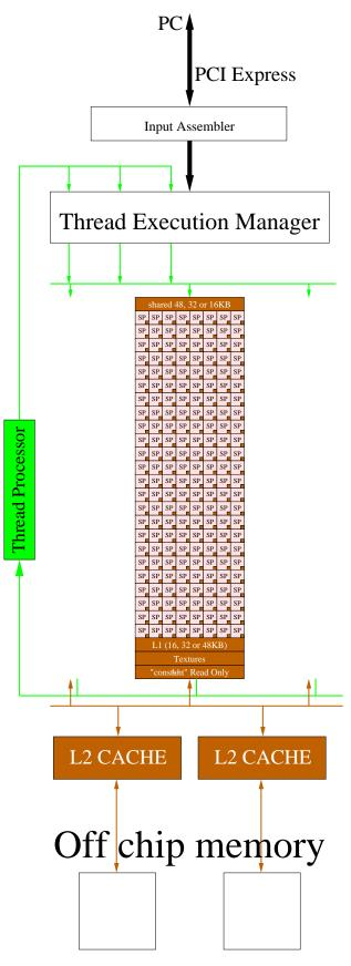
Fig. 4. Tesla K20c contains 13 SMX multiprocessors, a PCI interface to the host PC, thread handling logic and 4800 MBytes of on board memory. Each SMX contains 192 stream processors (only one SMX shown).
