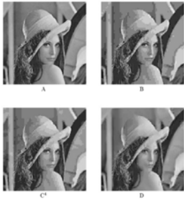
Fig. 5. Comparison between ERW, NN, and JPEG compression systems. A) Original Lena image. B) JPEG compression (bpp=0.3, SNR=26.2-26). C) NN compression (bpp=0.7, SNR=26.95). D) ERW compression (SNR=26.54, bpp=0.88).
