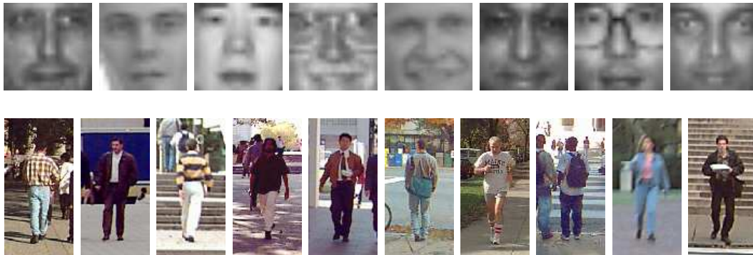
Figure 1: Top row : examples of images of faces in the training database. The images are 19x19 pixels in size. Bottom row : examples of images of people in the training database. The images are 128x64 pixels in size.
