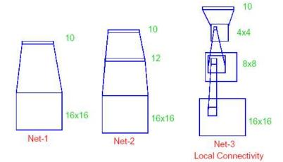
Local connectivity: each hidden unit is connected to only a subset of the units below it (specifically, in Net-3 in the 1st hidden layer, each unit connects to a 3x3 patch of the input layer; in the second layer inputs are 5x5 patches
