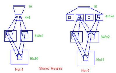
Net-5 is motivated by the fact that features of handwriting style should appear in more than one part of a digit. The weight sharing implement a form hard constraint on the weights
