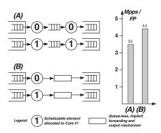
Fig. 5. 2-phase VS 1-phase forwarding mechanism
