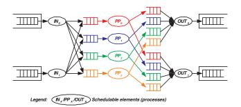
Fig. 3. Traditional software routers' forwarding architecture
