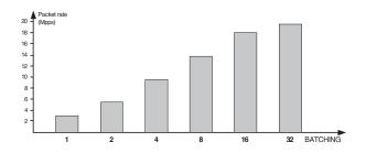
Fig. 11. The advantage of batch processing in software
