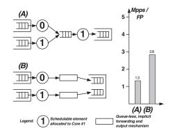
Fig. 6. Advantage of multiple transmit (Tx) queues
