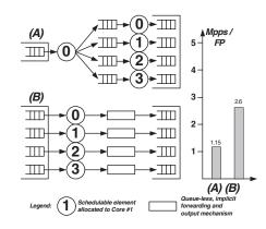
Fig. 7. Advantage of multiple receive (Rx) queues
