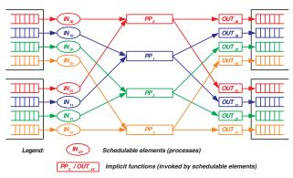
Fig. 4. Proposed software router forwarding architecture
