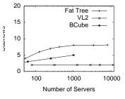
Figure 1: Throughput for long running connections using a permutation traf-<br/>fic matrix, for RLB and varying numbers of MPTCP subflowsFigure 2: Subflows needed to<br/>reach 90% network utilization
