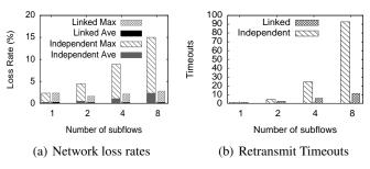
Figure 7: MPTCP vs. multiple independent TCP flows
