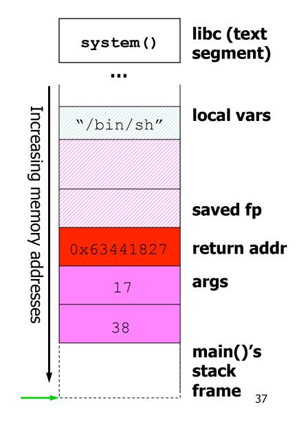
Instead of putting shellcode on stack, can put args there, overwrite return address with pointer to well known library function
