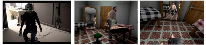
Figure 1 Left: a participant in motion capture suit, wearing a HMD; Middle:Avatar representation of the participant from third person view with mirror reflections and dynamic shadows; Right: First person view of avatar representation, with the avatar reflected in a mirror.
