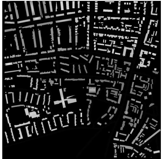
Figure 4: To find the reflected point (See figure 2) we perform a discrete ray tracing in a heightfield representation of the scene.
