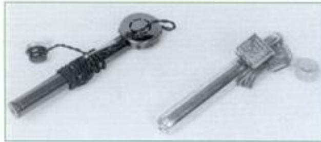
Figure 4. The Penfone at left and the Telex 300 were both hearing aids designed to look like fountain pens.
