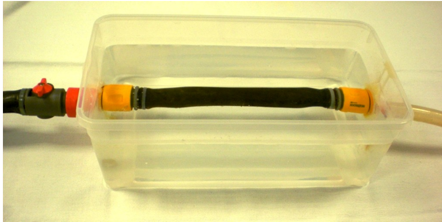
Figure 2.12: Photograph of rubber tubing vessel phantom used for in-vitro validation
