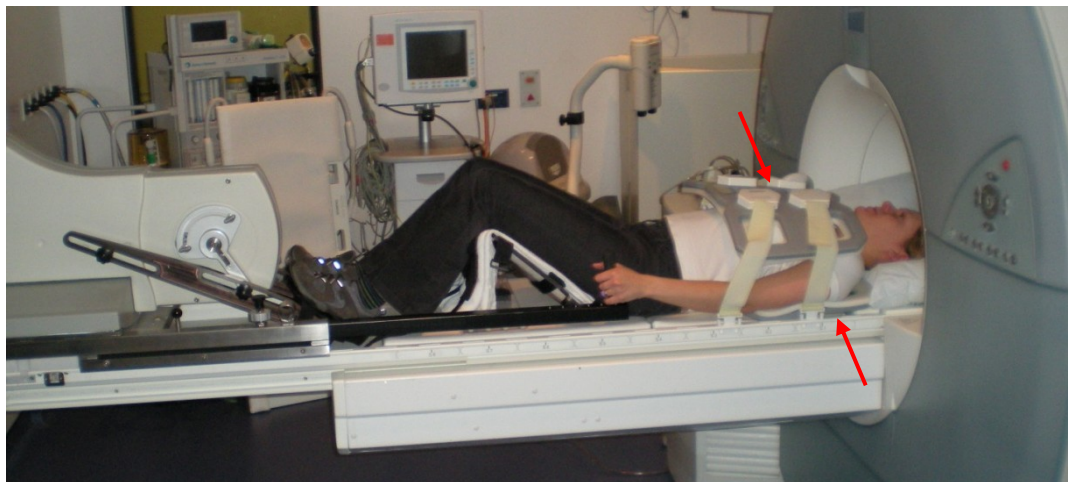
Figure 2.18: Coils used for imaging in-vivo; one body-matrix coil on top of the subject, and one underneath
