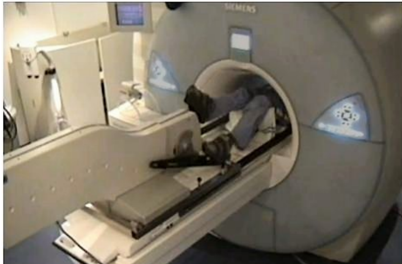
Figure 2.17: Photograph of a subject performing exercise on the ergometer, within the MRI scanner at ICH
