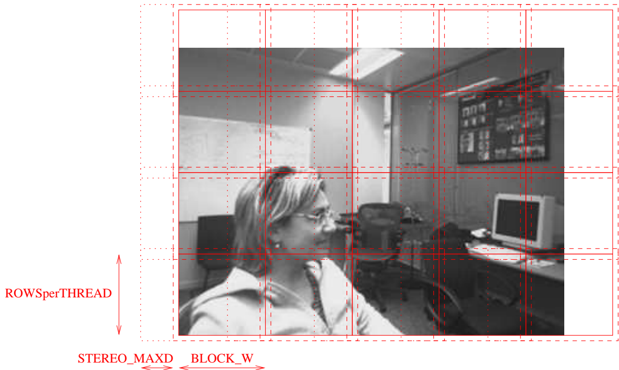
Figure 3: The left and right images (solid rectangle) are split into BLOCK\_W \times ROWSperTHREAD tiles. The dashed lines indicate the extra pixels outside the tile which must be read to calculate values for pixels in the tile. The right hand image is progressively offset by between zero and STEREO\_MAXD pixels (50, dotted lines).
