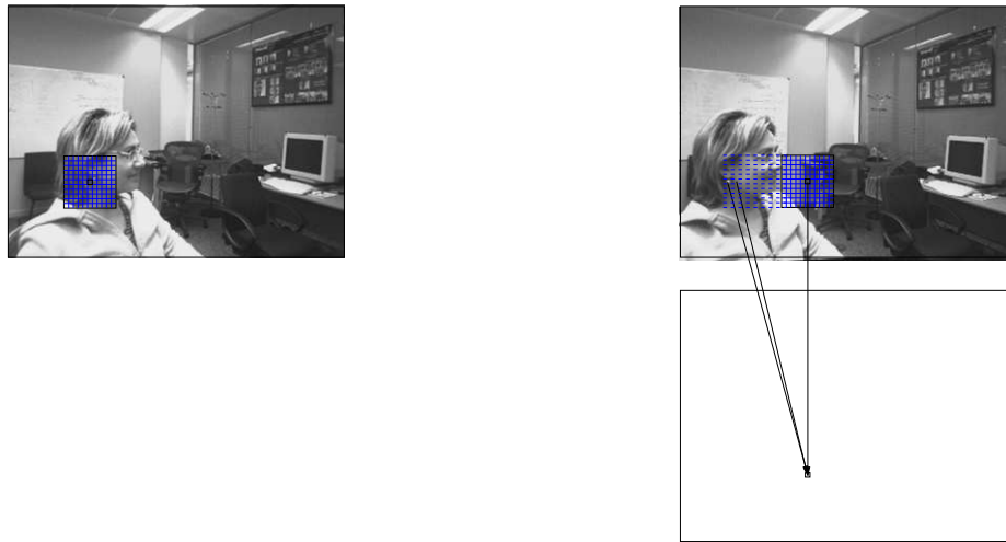
Figure 2: Schematic of stereo disparity calculation. Top: left and right stereo images. Bottom: output. Not to scale. For each pixel stereoKernel calculates the sum of squared differences (SSD) between 11 \times 11 regions centred on the pixel in the left image and the same pixel in the right hand image. This is the SSD for zero disparity. The right hand 11 \times 11 region is moved one place to the left and new SSD is calculated (SSD for 1 pixel of disparity). This is repeated 50 times. Each time a smaller SSD is found, it is saved. Although the output pixel (bottom) may be updated many times, its final value is the distance moved by the 11 \times 11 region which gives the smallest SSD. I.e. the distance between left and right images which gives the maximum similarity between them (across an 11 \times 11 region). This all has to be done for every pixel. Real time performance is obtained by parallel processing and reducing repeated calculations.
